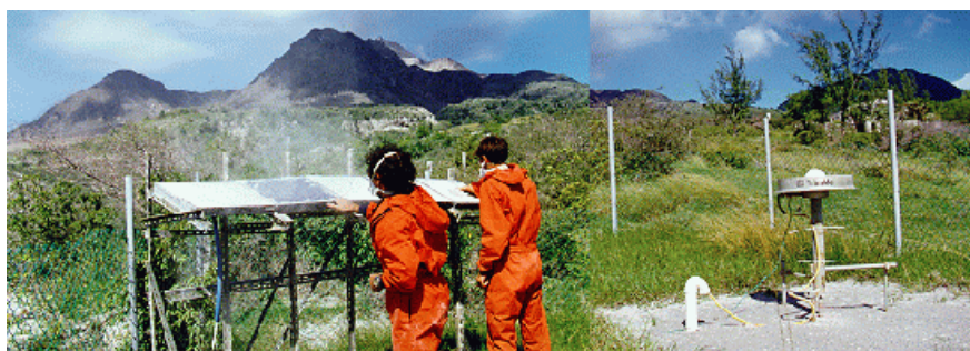
Figure 15 Applications of precise GPS measurements. Research into Earth processes via high-precision geodesy using GPS – A permanent GPS station collects remote measurements of surface deformation associated with volcanic processes (island of Montserrat, Soufrière Hills volcano) – image courtesy of UNAVCO (University NAVSTAR Consortium 1998) .
