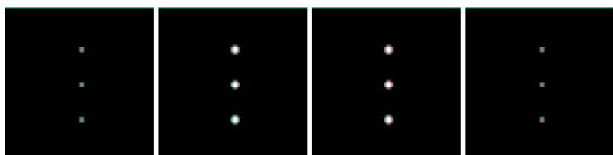
Fig. 2: Central slices of a 64 \times 64 \times 64 voxels phantom composed of three small spheres (radius = 1.75 voxel edge). The density of the voxel v_i is proportional to the volume of the voxel intersection with the small spheres (being equal to one when it is totally inside one of them). The image shows the planes perpendicular to the Y axis (the tilt axis is parallel to the Y axis).
