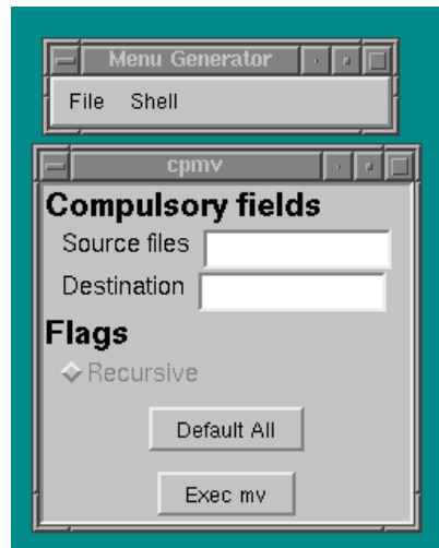
Figure 1. A screenshot for the simple copy and move interface. This window acts as a launcher for the appropriate copy and move commands: the source and destination files are selected by the user, and the command needed for that operation is run in a subshell when the 'Exec' button is pressed.
