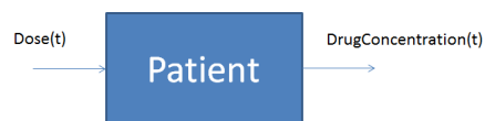
Figure 3.6: A patient can be regarded as a system that transform the signal corresponding to the drug doses into a plasma concentration of that drug.
