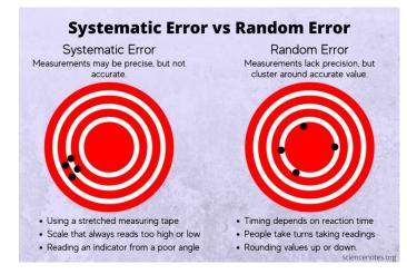
readings that differ from one reading to the next is an example of random error. The discrepancies between these readings and the real weight are due to the scale's random measuring inaccuracy.
