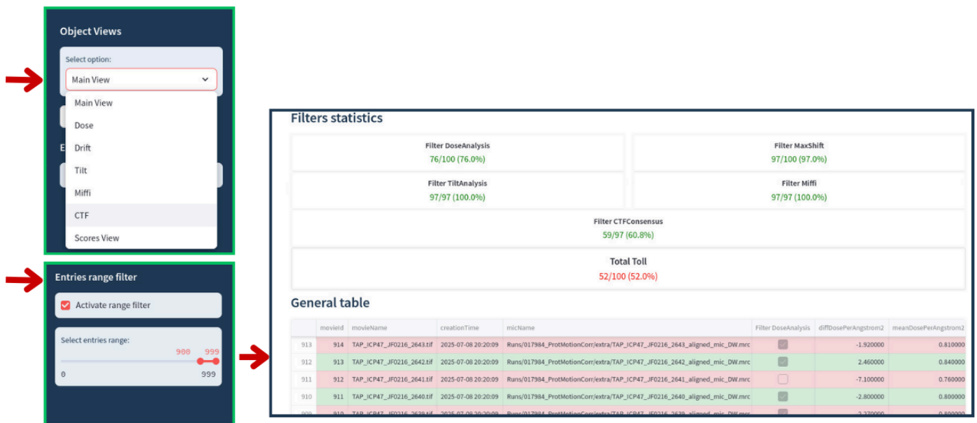
Figure 28. Interactive panels of the Main View. The Object Views and Entries Range Filter features are highlighted on the left with red arrows. The central white panel dynamically updates according to the user's interaction with these two features, displaying only the data or visual elements corresponding to the selected filter and entry range.
